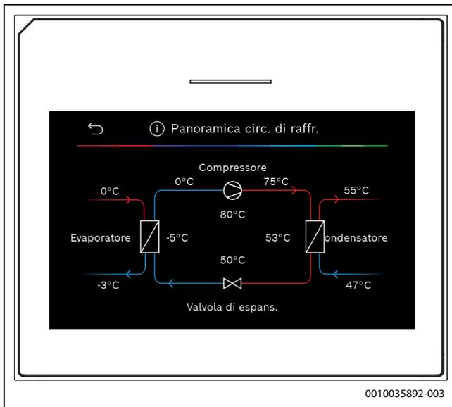
Fig. 10 Panoramic view of the refrigeration circuit
